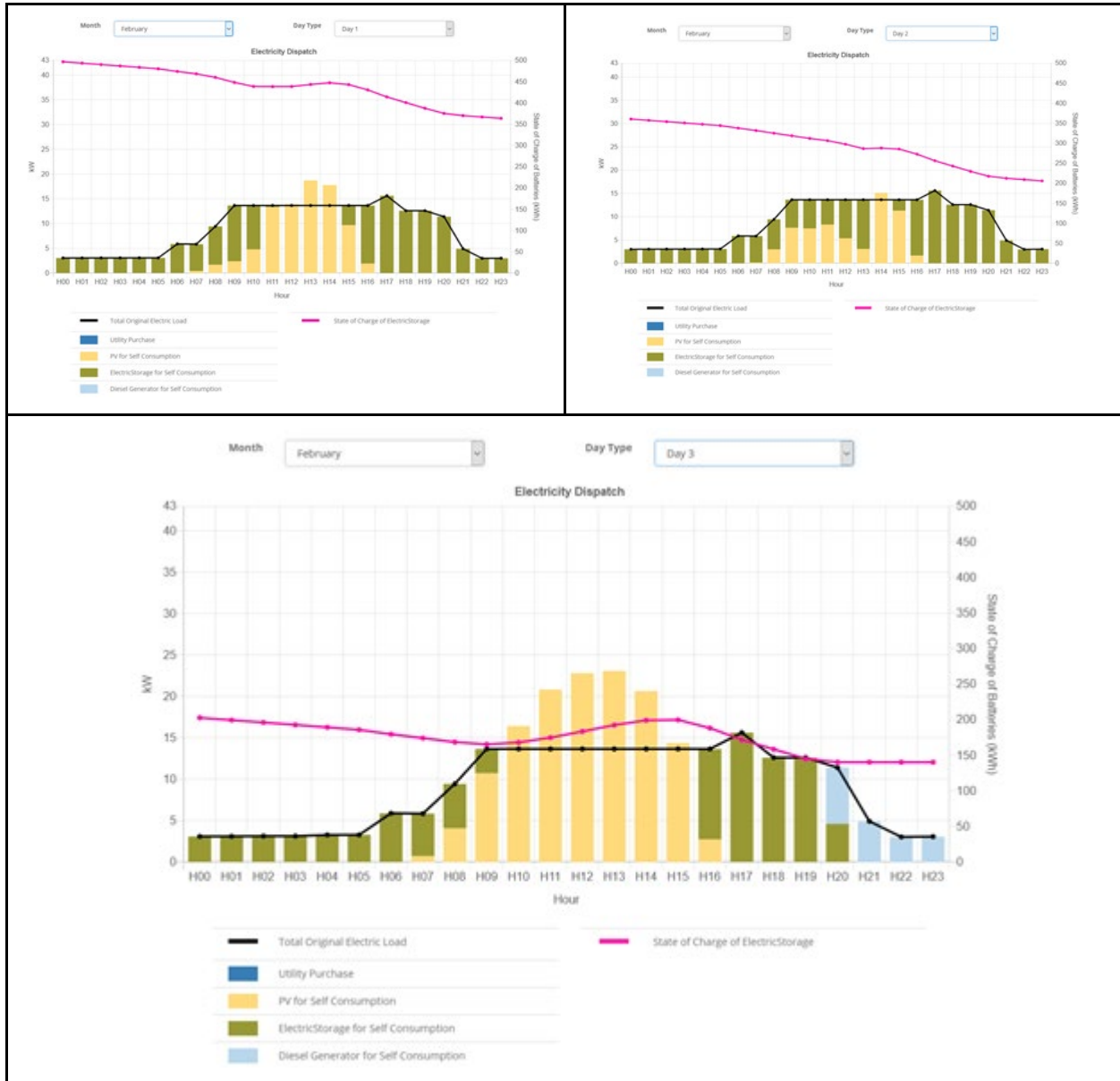
Figure A2: PSB outage scenario with 50% load (in each hour) and a forced 500 kWh battery. Left top figure represents the first outage day and it can be supplied completely with the battery (if some PV generation is available too). The right top figure represents the 2nd outage day and is also fully supplied with battery and PV power. Starting with the third day (bottom figure) the backup diesel generator needs to be used since the battery will be empty.
